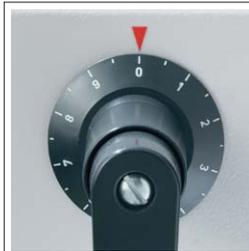
The calibrated hand crank and the measuring tape on the side lay ensure the exact positioning of the backgauge.
