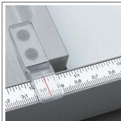
The accurate backgauge and side lays are made from cast aluminium and allow a precise alignment of the paper stack for exact cutting.
